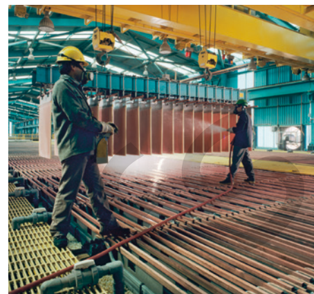
FIGURE 10.2.8 Plates of freshly deposited copper are removed from a copper electrorefining cell.
