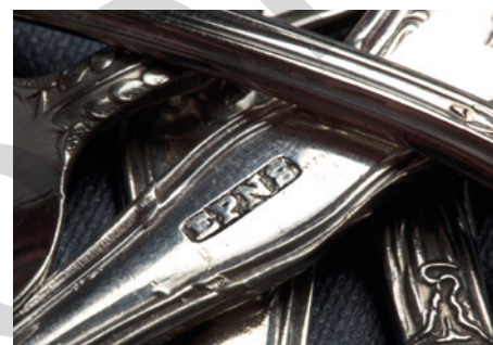
FIGURE 10.2.3 Silver electroplated cutlery. The letters EPNS stand for Electroplated Nickel Silver. Nickel silver is a copper alloy with nickel and often zinc that is used as the base metal for the cutlery.
