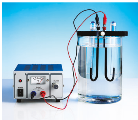
FIGURE 10.1.1 During electrolysis, electrical energy is used to make redox reactions occur. In this experiment, electricity passing through dilute sodium chloride solution creates bubbles of hydrogen gas at the left-hand electrode and bubbles of oxygen gas at the right-hand electrode. The gases are being collected in the test tubes.
